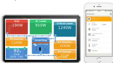
Visualization and system control via tablet, web portal and APP
